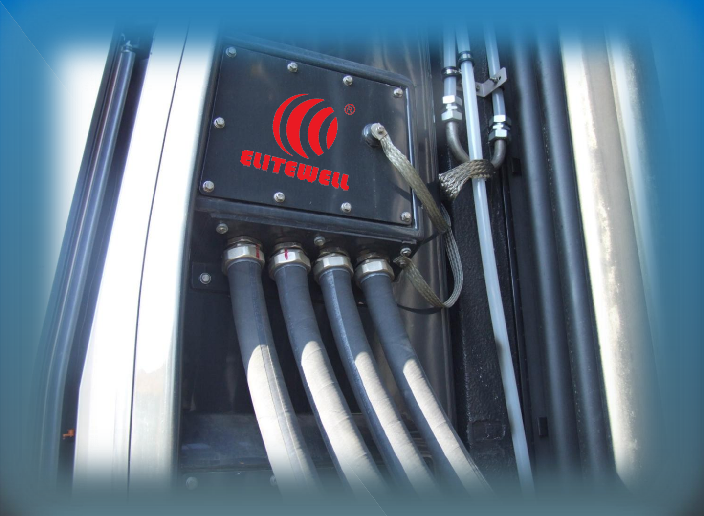
HV jumper cable as inter car body connection
