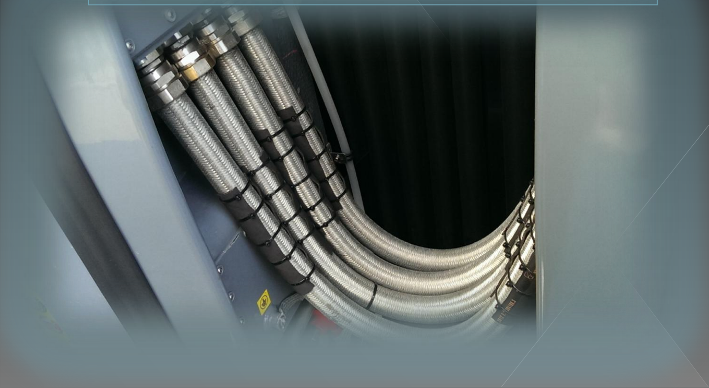
HV jumper cable as inter car body connection
